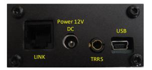
LINK – to connect to (1) Standard TelINF slave unit (6 pin modular connector / straight through cable)
